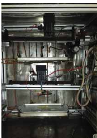
Fig. 1. Integrated electro-spray freeze drying system-(pilot scale facility for nano-particles production)
