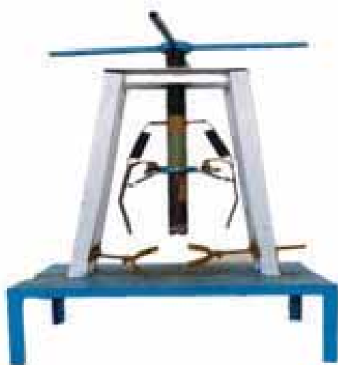
Fig. 1. Jackfruit coring and peeling machine
