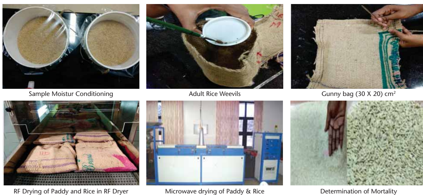
Fig. 1. Mortality study of paddy & rice in Radiofrequency & Microwave treatment
